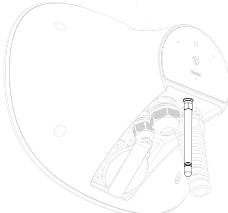
3. Insert the ethernet cable through the data cable entry\*.
