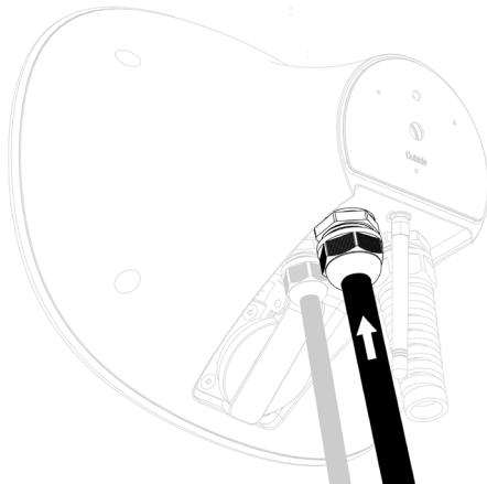
5. Retighten the cable entry nut (2 Nm).
