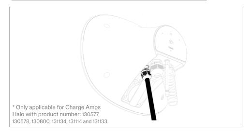
4. Strip the power cable (15-20 cm) and insert through the power cable entry.
