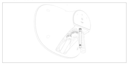
3. Insert the ethernet cable through the data cable entry\*.
