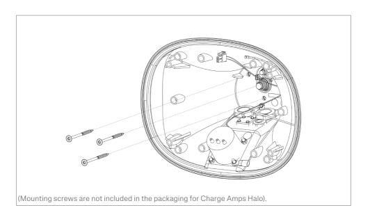
8. Mark and drill mounting holes on the wall for the Vehicle connector holder. Place the holes for the Vehicle connector holder approximately 30 cm to the right of Charge Amps Halo.
