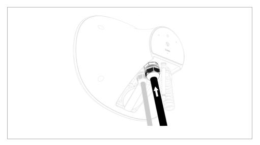
5. Retighten the cable entry nut (2 Nm).
