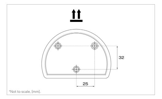
7. Mount the back cover on to the wall. Make sure the mounting surface is vertical and flat.
