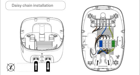
N.B: Make sure the cables are straight after the cable gland to avoid strain on the cable glands and plastic parts. Important! Make sure to cover non used cable entries with suitable plugs found in the Accessories kit.
