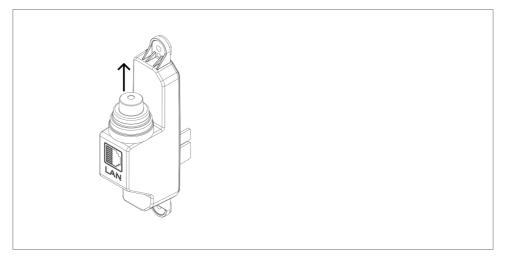
3. Make a hole in the rubber grommmet using a screwdriver or similar.
