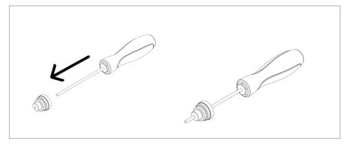
4. Pull the rubber grommet over the LAN cable and mount the RJ45 plug to the LAN cable.
