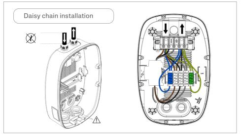
Important! Make sure to cover non used cable entries with suitable plugs found in the Accessories kit.
