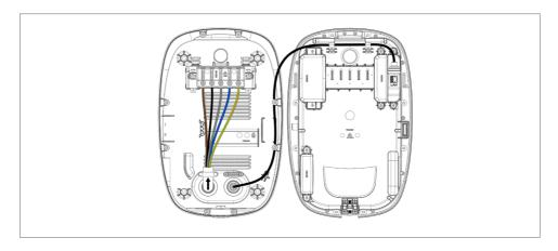
2. Remove the rubber grommet from the LAN module.
