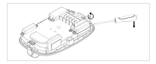
2. Mount the LAN module and screw it in place. Attach the cable clips using the screws included in the packaging.
