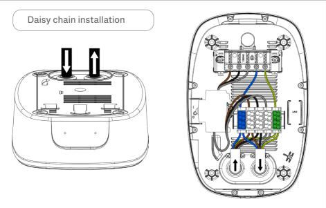
Important! Make sure to cover non used cable entries with suitable plugs found in the Accessories kit.
